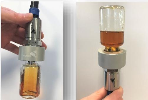
Step 5: Carry out a visual check by selecting the bottle that most closely resembles state of the oil sample.
