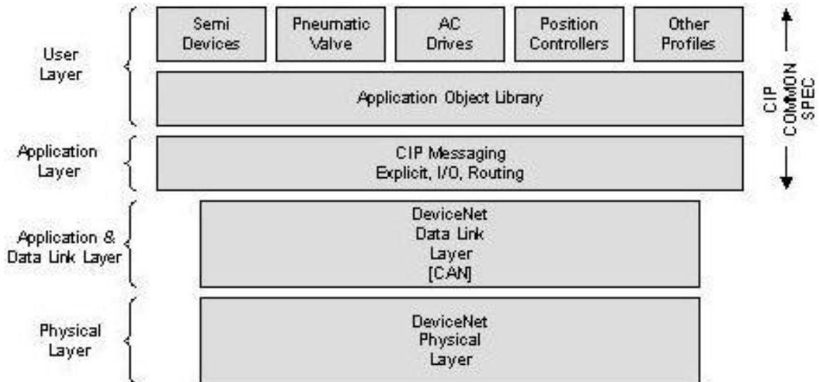
The DeviceNet™ specification defines the Application Layer and the Physical Layer. The Data Link layer is based on the CAN-specification. For the optimal industrial control will be defined two different messaging types. I/O messaging (Implicit Messaging ) and explicit messaging. With Implicit Messaging becoming I/O data exchanged in realtime and with Explicit Messaging becoming data exchanged to configure a device.
