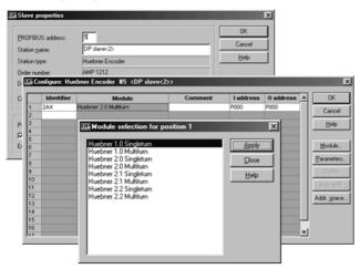
Now select the profile for the encoder operation. The input and output address are then assigned, and the parameterization can be carried out. This function can be called up by the PARAMETERS button in the CONFIGURE window, and provides a clear and simple way of setting the parameters.
