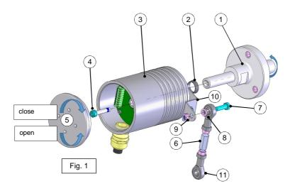
1. Mount adapter shaft (1) and align using dial gauge.
