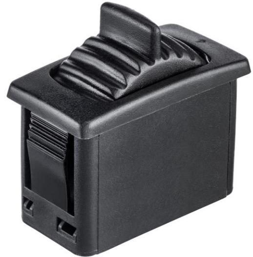
The JC050 is a roller for use in joystick grips and other in-cab human-machine interfaces. A robust, return-to-center mechanism provides movement over a range of  $\pm 37^\circ$ , with the thumbwheel having an option of a lever profile to ease operation. A compact mechanical design means the required under-panel space is just 23mm.
