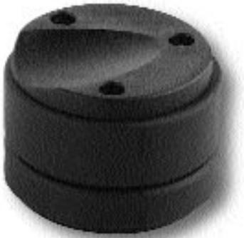
The SWR is a compact switched rocker offering finger tip/thumb control in up to 4 half axes. The unit is supplied with an 'O' ring so as to ensure IP66 sealing above the panel and is capable of switching a resistive load of up to 100mA.
