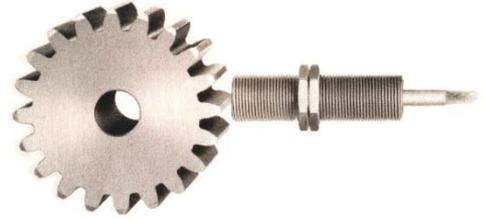
These sensors comply with the NAMUR standard respectively to DIN 19234 and can also be mounted in hazardous areas, as long as they are connected to intrinsically safe circuits. The measuring principle of these sensors is based on the fact that the measured object, which can consist of any type of metal, extracts more or less energy from a transistor oscillator, thus bringing about a variation in the current consumption.
