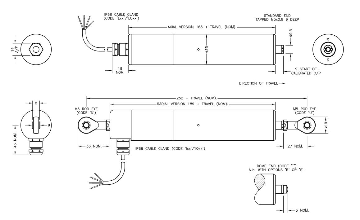
MAXIMUM WORKING DEPTH: 100 METRES/328 FEET. WHERE THE FREE END OF THE CABLE IS TO BE TERMINATED IN A SUBMERGED POSITION, ADEQUATE SEALING MUST BE PROVIDED TO PROTECT CONNECTIONS. THE PUSH-ROD RETRACTS A FURTHER 4mm NOM. FROM START OF CALIBRATED TRAVEL. STANDARD VERSIONS THE PUSH-ROD EXTENDS A FURTHER 8mm NOM. FROM END OF CALIBRATED TRAVEL, FOR SPRUNG VERSIONS: 'R': 1mm, 'S': 2mm. 'V' CODED PUSH-ROD WILL DEPART SENSOR BODY.
