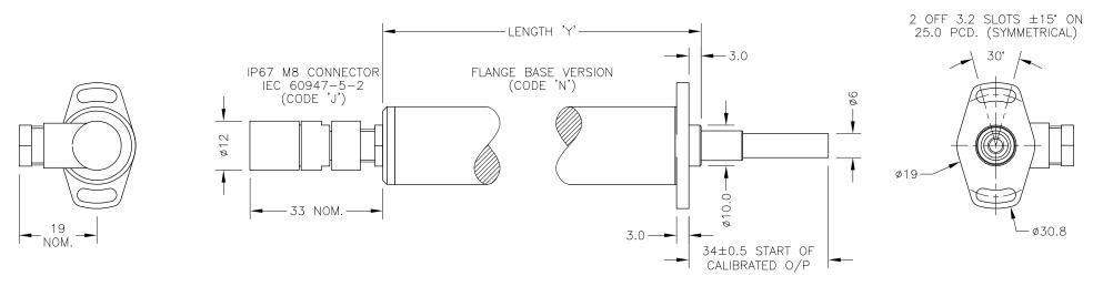
DOME END\* (CODE 'T') R7.0 (SPHERICAL)
