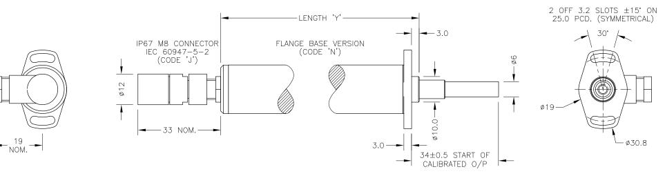
NOTE: SENSORS ARE MADE IN FOUR STANDARD LENGTHS. TRAVEL: (mm) BODY LENGTH: (mm) 'Y' FLANGE CALIBRATED MECHANICAL 'X' <u>STANDARD</u> 0-51 TO 0-70 70 138.0 132.5 0-71 TO 0-100 100 162.5 168.0
