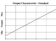
Retracted Linear Displacement Extended
