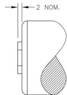
\*HOUSING BORE TO SUIT PROBE: Ø20.10 TO Ø20.15
