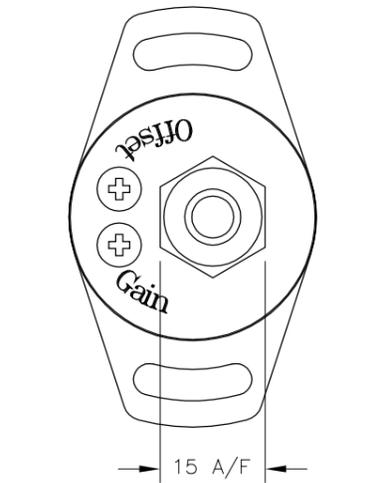
GAIN AND OFFSET ADJUSTMENTS SEALED (CODE 'Y')
