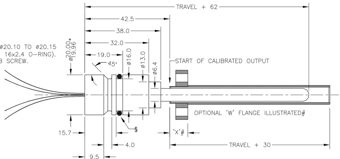
CONNECTIONS BETWEEN PROBE AND ELECTRONICS MODULE: FOUR WIRES; RED, BLACK, GREEN AND YELLOW, LENGTH: 300, CROSS SECTION: 0.25mm<sup>2</sup>, WIRES POTTED IN PROBE HOUSING. INTERCONNECTIONS MUST BE PROTECTED FROM WATER INGRESS AND STRAIN RELIEVED.
