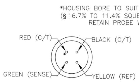
\*HOUSING BORE TO SUIT PROBE:  $\phi 20.10$  TO  $\phi 20.15$  (§ 16.7% TO 11.4% SQUEEZE WITH 16x2.4 O-RING). RETAIN PROBE WITH GRUB SCREW.
