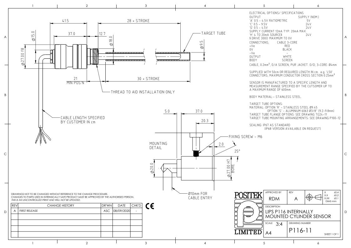
TARGET TUBE OPTION NOTES:-1. SPECIFY TUBE MATERIAL; CODE:-'R' STAINLESS STEEL 316 Ø9.45.
