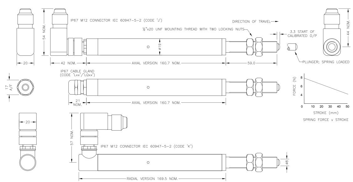
SUPPLY CURRENT 12mA TYP. 20mA MAX. CABLE: 0.2mm², O/A SCREEN, PUR JACKET — SUPPLIED WITH 50cm OR REQUIRED LENGTH IN cm (15000cm MAX). STANDARD 3—CORE: JACKET Ø4mm BLACK e.g. 'L50' OPTIONAL 5-CORE: JACKET Ø4.6mm BLUE e.g. 'LQ50' CABLE/CONNECTOR\* CONNECTIONS; 3 CORE 5 CORE CONNECTOR RED RED ORG +SENSE (5-WIRE ONLY) :1 BLACK BLACK :3 OV GRY -SENSE (5-WIRE ONLY) WHITE WHITE OUTPUT SCREEN SCREEN :4 BODY
