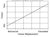
**Output Characteristic:** Plunger extended 28 mm<sup>\*</sup> from mounting face at start of normal travel. \*Note: where dome end option is fitted add 5 mm.
