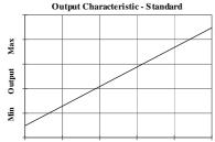
Retracted Linear Displacement Extended
