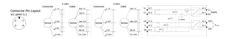
Approval only applies to specified ambient temperature range and atmospheric conditions in the range: 0.80 to 1.10 Bar, oxygen  $\leq$  21%. The H133 is available with the following connections:-
