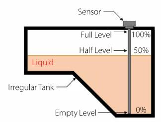
In this situation, 50% of tank volume is not half way up the probe. To correct for this tank profiling can be used. This can be done in the GSlevel software and is covered in detail in the GSlevel User Manual.
