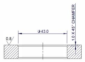
Fit the gasket over the thread mount, black face up. Ensure the gasket is centred under the sensor and tighten the sensor using a 59.5 mm A/F spanner to a torque of 50 Nm.
