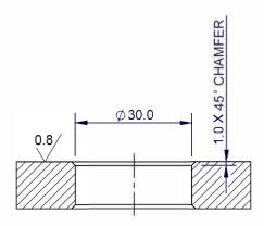
Fit the gasket over the thread mount, black face up. Ensure the gasket is centred under the sensor and tighten the sensor using a 59.5 mm A/F spanner to a torque of 50 Nm.
