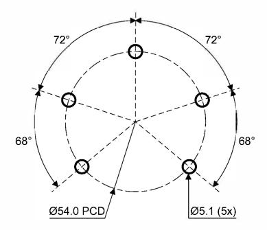
The sensor should be fitted with a gasket if the SAE 5-bolt installation method is used. Fit the gasket over the bolts, black face up, and tighten the bolts to a torque of 10 Nm each.
