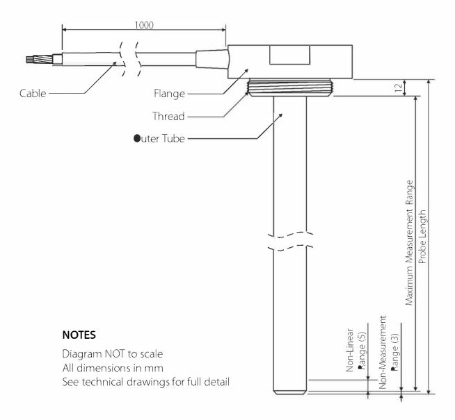
The sensor electronics are housed in the flange, outside the measurement tank. The outer tube is placed into the measurement tank, such that will be submerged in liquid. The sensor can be installed using either built in thread or a five bolt SAE mounting, both providing a tank seal.
