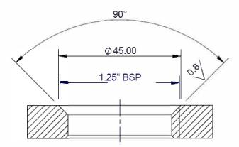
Fit the O-ring above the male thread on the sensor. Ensure the O-ring is centred and sits within the chamfer; tighten the sensor using a 59.5 mm A/F spanner until the sensor face is flush with the top of the tank and a torque of 50 Nm is achieved.
