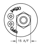
GAIN AND OFFSET ADJUSTMENTS SEALED (CODE 'Y')
