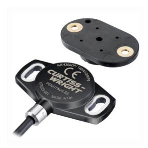
The NRH300DP is a no-contact, Rotary Position Sensor that offers the optimal combination of performance, safety and cost. The sensor utilises proven Hall-effect, sensing technology in a low-profile (8mm) housing with separate magnet for true no-contact sensing.
