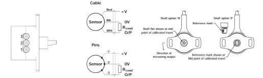
Mechanical Mounting: Flange mounted. The flange slots are 4.5mm by 20 degrees wide, 48mm pitch. The sensor should be mounted with minimal axial and radial loading on the shaft for optimum life. It is recommended that the shaft is coupled to the drive using a flexible coupling. Option 'N' shaft:  $\emptyset$  4 mm x 8 mm long, flat 3 mm A/F x 4 mm. Option 'P' shaft: fits 6 x 3 mm slot.
