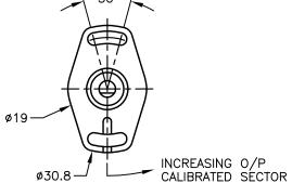
SHAFT FLAT ALIGNED WITH REFERENCE MARK IN BASE AT MID TRAVEL ±5"
