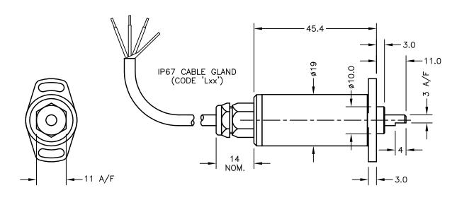
FLANGE BASE (STANDARD) 2 OFF 3.2 SLOTS ±15° ON 25.0 PCD. (SYMMETRICAL)
