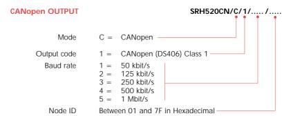
Baud rate and Node ID are initially set at the factory before despatch.
