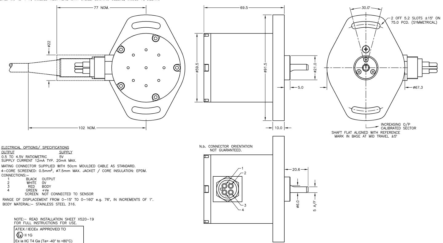
UI 11.4V, II 0.2A, PI 0.51W APPROVED FOR USE IN CONJUNCTION WITH A GALVANICALLY ISOLATED BARRIER.
