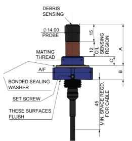
The WearDetect provides continuous real-time monitoring of ferrous debris that it captures from the lubricating oil.
