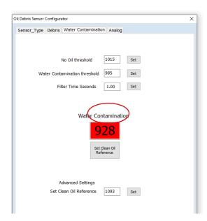
Select 'Set Water Contamination Reference' and the Water Contamination window will return to green.
