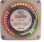
Red (Flashing) -Maximum debris condition breached
