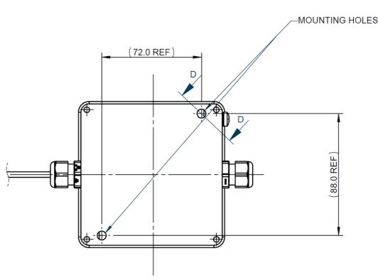
Two 4.2mm diameter mounting slots are provided for fixing the electronics enclosure to a fixed surface. The fixings must be suitable for supporting the weight of the enclosure. The following figure shows the mounting dimensions:
