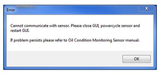
Check the cable is correctly inserted at both ends and that the sensor is powered. It is also possible that the installation of the device drivers has not yet been completed. Re-starting usually clears the problem. If not, then check that sufficient power is being supplied to the sensor.
