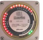
Red (Flashing) -Maximum debris condition breached
