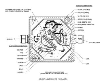
Fit wires with the bootlace ferrules provided prior to termination into the terminal block.
