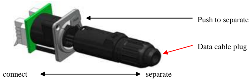
Figure 7-6 Connection of Data Cable with Handset
