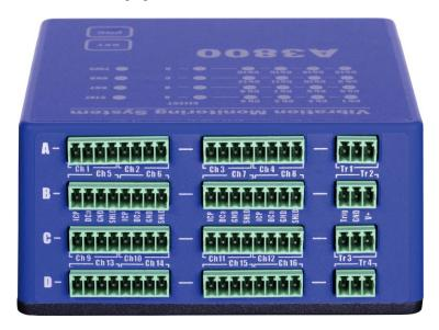
The connectors for connecting the sensors are located on the top panel. Connectors are divided into groups A, B, C, D.
