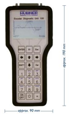
All measured data will be stored in the device. By means of the USB interface the measured data can be transferred to a PC/Laptop and further analyzed there with the supplied software.
