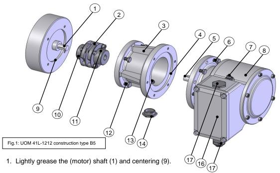
2. Fit coupling (2) onto (motor) shaft.
