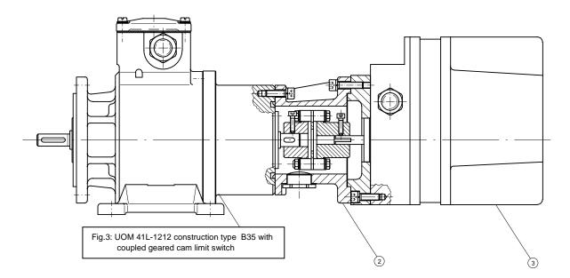
When supplied ex works the second shaft end is protected by a cover plate
