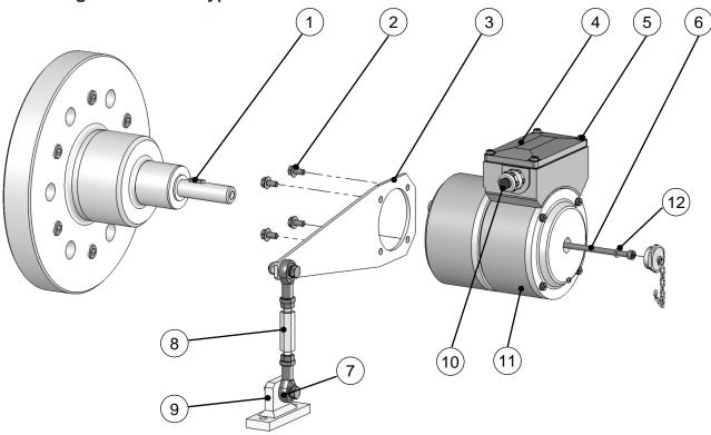
1. Mount adapter shaft (1) and align using dial gauge.
