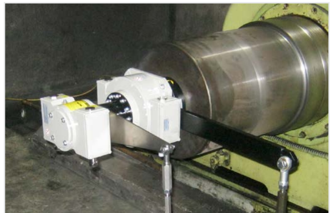
A series 41 safety encoder in combination with a standard encoder (e. g. series 6/60).
