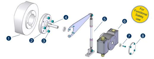
Example 2: A series 41 safety encoder in combination with a standard encoder (e.g. series 6/60)
