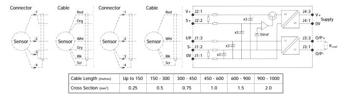
To ensure correct operation of both Amplifier and sensor, the following restrictions on conductor cross section and cable length limits are set out in the table above (figures are based on copper conductors);
