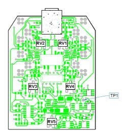
To calibrate the temperature output for a module configured for a  $10\text{mV}/^{\circ}\text{C}$  sensor, the milliammeter is connected to terminals M and J. With no input signal applied the output current can be set to 4.0mA using potentiometer RV2. A dc voltage corresponding to the maximum temperature (eg.  $1.0\text{V} = 100^{\circ}\text{C}$ ) is then applied to terminals C and F. The output current can then be adjusted to the maximum 20.0mA using potentiometer RV4.
